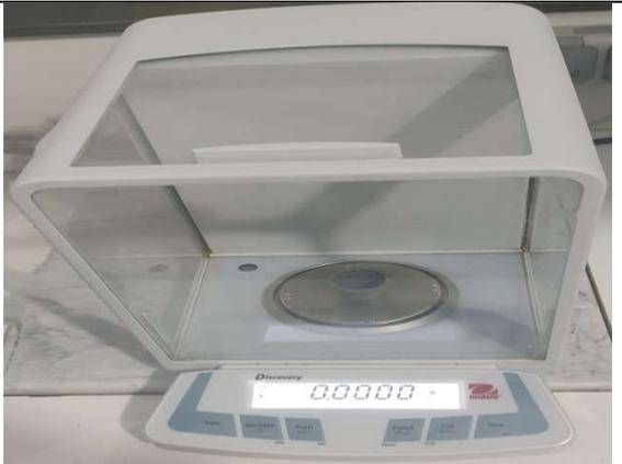
A white Ohaus precision balance with a stainless steel weighing pan and a digital display showing 0.0000.           | Balance de précision |
