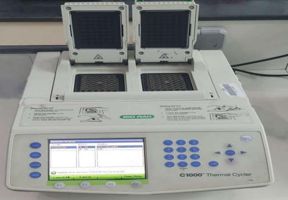
A white Bio-Rad C1000 Thermal Cycler with two sample blocks and a digital display showing a PCR protocol.             | Thermocycleur        |
